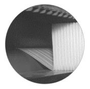
Conventional mini-pleat media packs are produced by taking a roll of media and using either glue, strings, or strips of media as a separator. The media pack is pleated, and the separators give the media pack its shape and strength.
